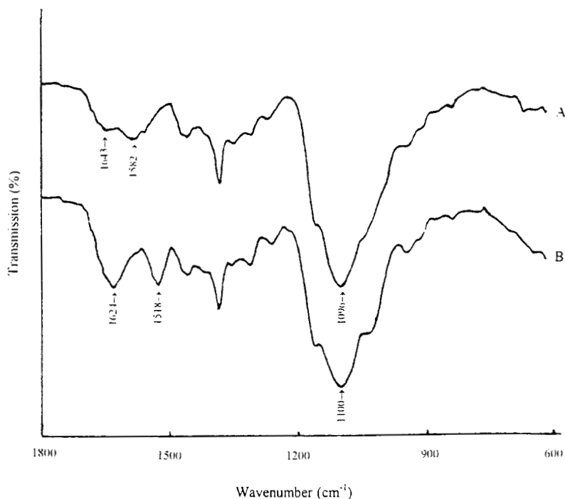
Figure 2 IR spectra of dry gels: (A) chitosan-polyether semi-IPN and (B) IPN swollen in pH = 1.25 medium.
